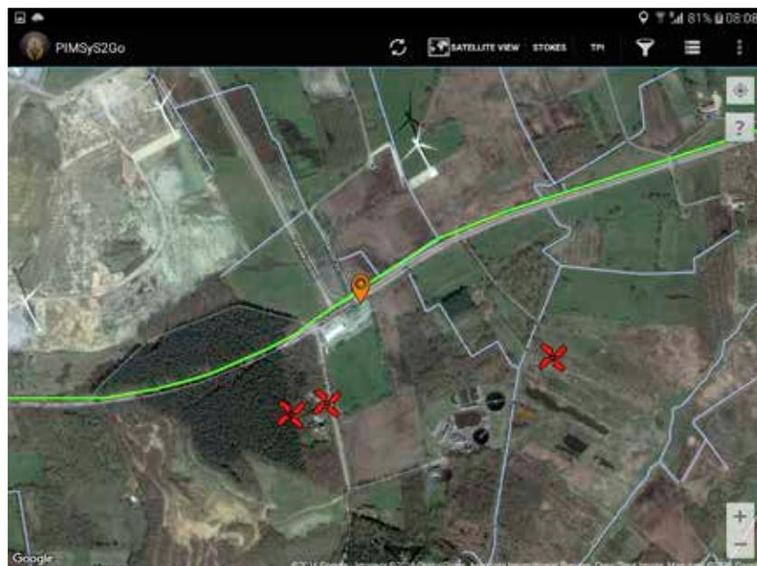
Figure 1. A mobile device using the PIMSyS app that is showing the pipeline route (green line), a TPI notification detected by PIMSyS (orange placeholder) and helicopter reports (red rotor blades).
