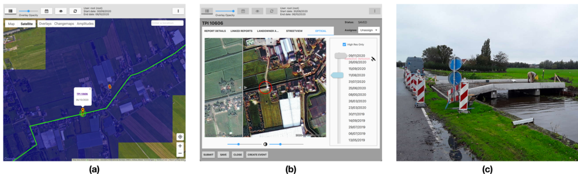
Figure 2: Detection and follow-up of a TPI: (a) a detected anomaly is shown on the map interfering with the pipeline corridor, (b) using high-resolution optical data the location of the TPI can be analyzed and (c) a field inspection is done to verify the activity and take mitigating measures when appropriate.
